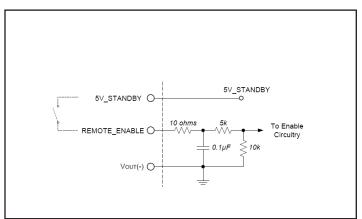
Figure B: Remote enable interface circuitry.
