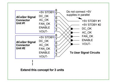
Figure P2: Simplest Signal Connections
