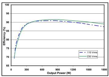
Figure 3: 15 VOUT efficiency curves.
