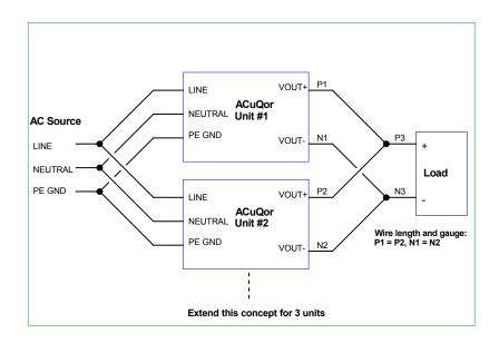
Figure P1: Parallel Power Connections
