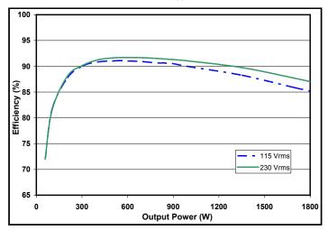
Figure 1: 12 VOUT efficiency curves.
