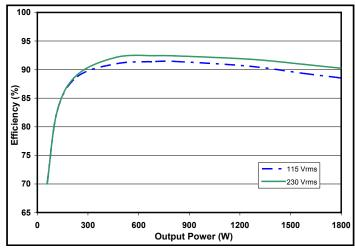
Figure 7: 28 VOUT efficiency curves.
