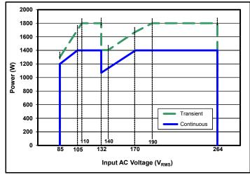
Figure 12: Rated output power vs Input AC Voltage.
