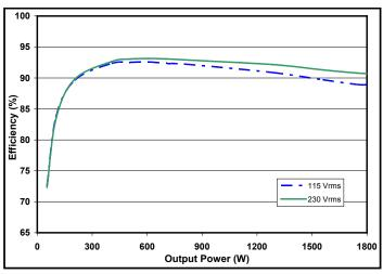
Figure 9: 48 VOUT efficiency curves.
