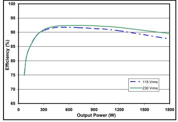
Figure 5: 24 VOUT efficiency curves
