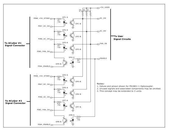
Figure P4: Isolated Signal Connections
